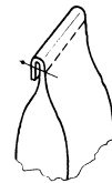
Fold-over closure manually by operator or by additional bag feed-in device with bag-top fold-over device
